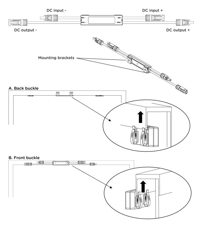
NOTE: Do not place the RSD-S-PLC (including DC connectors) where exposed to the sun, rain or snow, even gap between modules. Allow a minimum of 3/4"(1.5cm.) between the roof and the bottom of the RSD-S-PLC to allow proper air flow.
