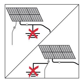
The inverter is designed exclusively for connection to and use with non-grounded solar modules. The solar modules must not be grounded at either the positive or negative pole.
