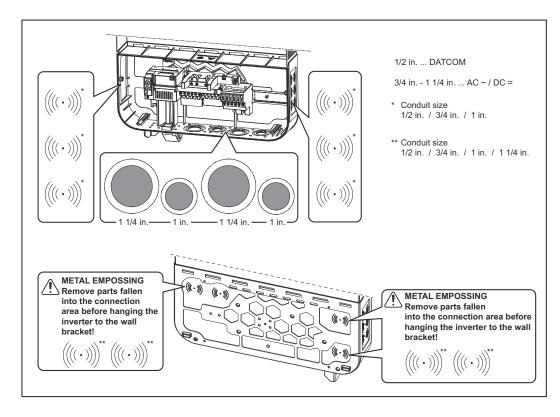
The wall bracket contains several knockouts of different sizes. When knocked out, the openings are used for the inputs of various wires.
