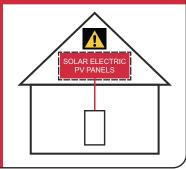
**Warning!** The installer is responsible for the correct labeling of the PV system. The rapid shutdown requirement of the inverter is not affected by the FRT (fault ride through) capability, so the inverter is "Grid support interactive compatible"
