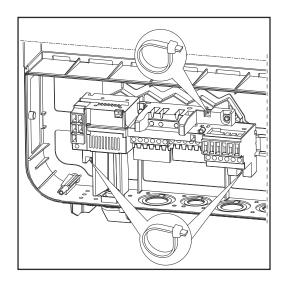
If excessively long AC or DC cables are laid in loops in the connection area, fix the cables to the designated eyelets at the top and bottom of the connection block using cable ties.
