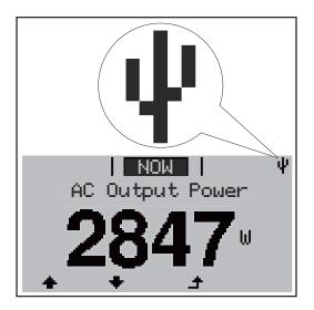
When the inverter recognizes a USB thumb drive, the USB symbol will appear at the top right of the display.
