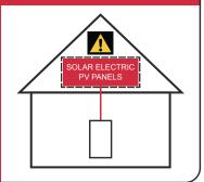
In case a string-level shutdown equipment at the PV array is used in combination with the inverter, this labeling has to be used according to NEC (Section 690.12), CEC (64-218).
