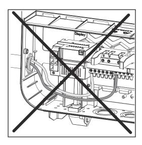
If DC cables are laid over the shaft of the DC main switch or across the DC main switch connection block, the cables may be damaged when the inverter is pivoted or the inverter may not be able to be pivoted.
