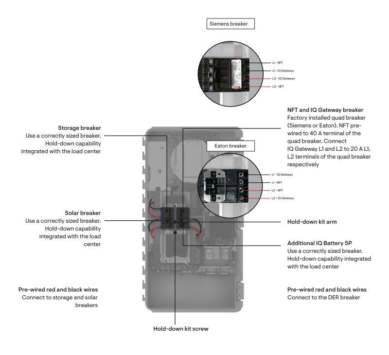
Figure 1B: Installing DER breakers for IQ8 System with generator
