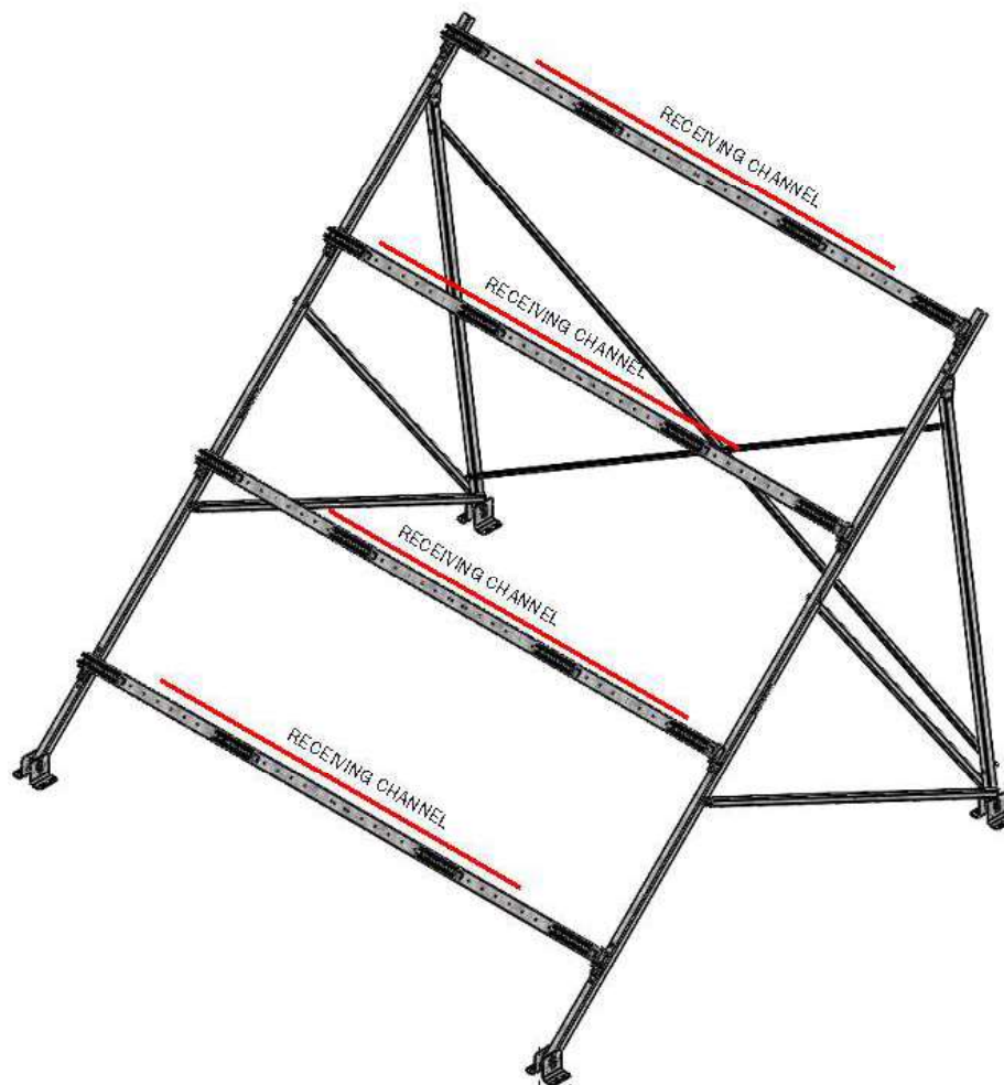
Image 19: Typical 6 Module Steel Tube Rail Installation Shown
