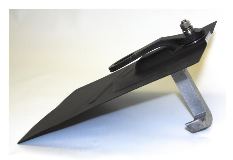
The device consists of a "J-hook that hooks under a timber rafter or top chord member of a timber truss through a hole drilled in the roof sheathing beside the rafter or top chord member. After installation of the "J-hook" and upper plate, flashing is installed over the roof penetration and a rotating lug is bolted to the "J-hook" to allow a worker to connect their body harness lanyard to the anchor.
