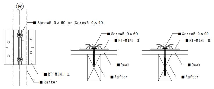
2 Rafter installation (Offset) : Fastened to the Rafter offset with 2ea. M5.0  $\times$  60 mm wood screws on either side and 3ea. M5.0  $\times$  60 mm wood screws to the sheathing.
