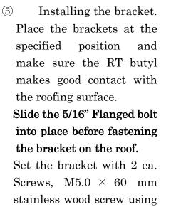
After completing process, make sure the brackets are securely fixed.
