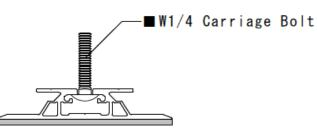
Note: M8 and M6 Bolt will not fit the RT-MINI II base.
