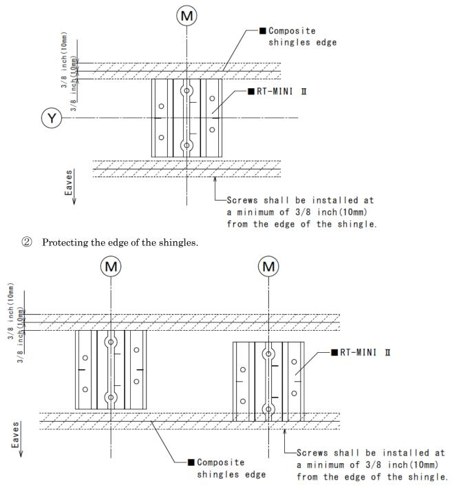
① Locate and place MINI II base on the cross section of chalk line.
