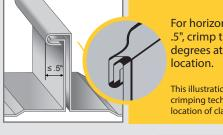
For horizontal seams under .5", crimp the seam to 180 degrees at desired clamp location.
